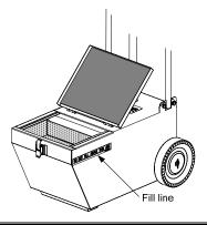
4. Carefully withdraw the unit far enough to allow the cover to be closed. Latch the cover in the closed postion. Using the handle, carefully tip the unit back slightly for ease of handling and roll the unit to the disposal site.
